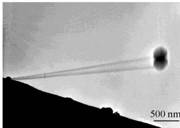
Figure 5. Measurement the work function of an attached carbon particle on the tip of a ZnO nanobelt at f = 0.349 MHz and V_{ac} = 9.0 V.
