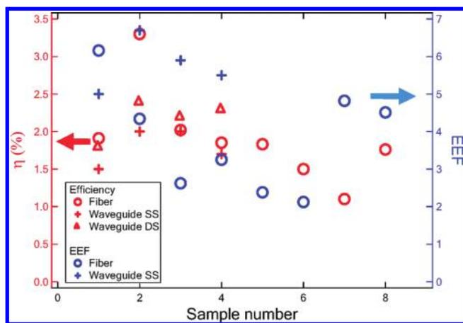
FIGURE 4. Comparison of energy conversion efficiencies and efficiency enhancement factors ( $EEF = \eta_{PS}/\eta_{NS}$ ) of planar waveguide–NW and fiber–NW<sup>12</sup> 3D DSSCs.
