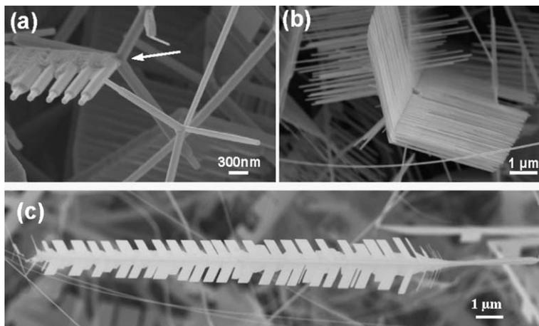
Fig. 4. (a) A single-sided nanocomb ending with a tetra-leg structure. (b) and (c) feather-like double-sided nanocombs with an angle of  $\sim 110^\circ$  between the two sides.
