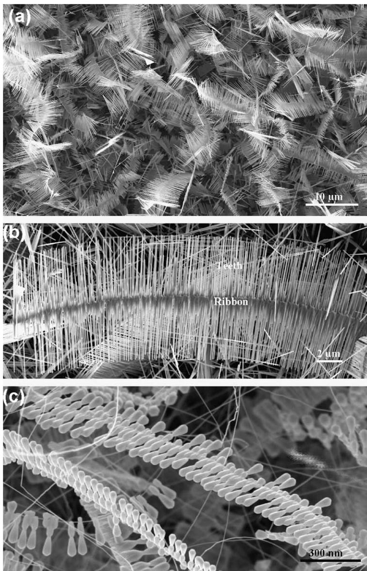
Fig. 2. SEM images of the double-side teathed ZnO comb structures. (a) A low magnification SEM image showing the high yield of the symmetric combs. (b) and (c) double-sided ZnO nanocombs with different morphologies.
