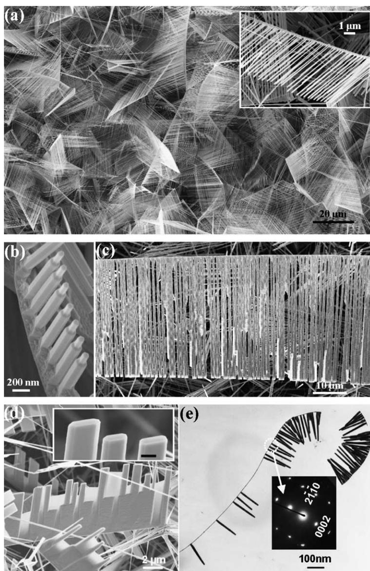
Fig. 1. (a) As-grown, single-side teathed ZnO comb structures. Inset is a magnified image of a single-sided comb; (b) to (d) are SEM images of single-sided combs with different morphologies. (e) A typical TEM image of the single-sided nanocomb. Inset diffraction pattern is from the circled area showing that the growth direction of the teeth is  $[0001]$ .
