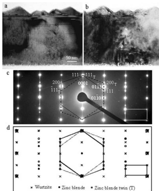
Fig. 5. a,b) TEM images of a saw-like ZnS nanostructure prior and after illumination by an electron beam for ca. 10 min, showing the formation of planar defects. c) Electron diffraction pattern recorded from the area which can be indexed as the coexistence of the hexagonal and cubic phases with the presence of twins in the cubic phase. d) A schematic showing the systematic reflections in corresponding to the experimental pattern shown in (c).
