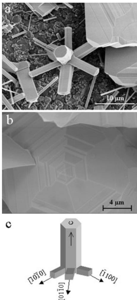
Fig. 4. a) SEM image of the windmill structure. b) SEM image of the polyhedral structure of ZnS. c) Structural model of the windmill structure.
