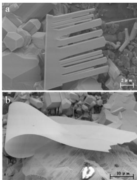
Fig. 2. SEM images of ZnS comb-like and sheet-like structures.
