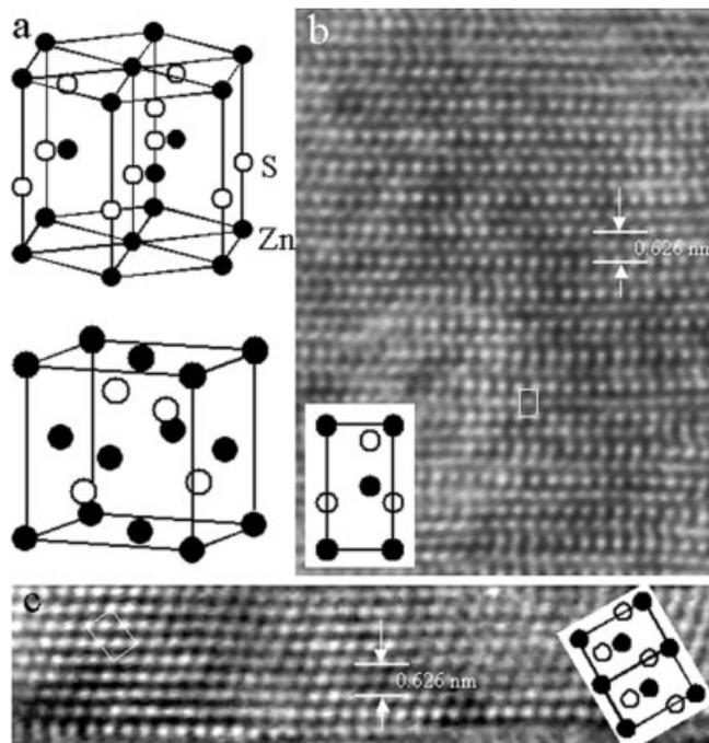
Fig. 6. a) Unit-cell models for the hexagonal and cubic phases. b)  $[2\bar{1}\bar{1}0]$  High-resolution TEM image of the wurtzite ZnS. c)  $[01\bar{1}]$  High-resolution TEM image of the zinc blende ZnS. The insets are the projections of the corresponding unit cells.
