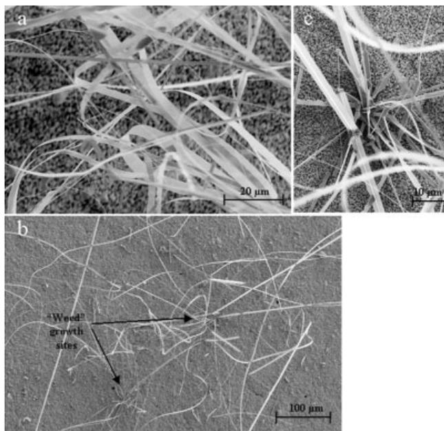
Fig. 1. a) SEM image of ZnS nanobelts and nanosaws grown from an alumina substrate. b,c) Distribution of the ZnS nanobelts on the substrate surface suggesting a “weed growth” model.
