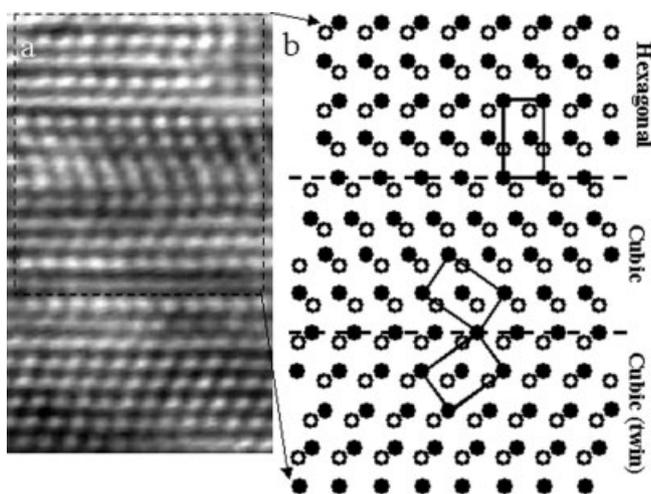
Fig. 7. High-resolution TEM image showing the coexistence of the wurtzite, zinc blende, and the twinned zinc-blend structures; the corresponding structure model is illustrated at the right-hand side showing the transformation among the structures by adjusting the stacking sequence of the atomic layers.
