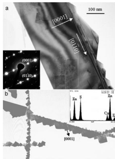
Fig. 3. a) TEM image and the corresponding electron diffraction pattern from a belt- and saw-like ZnS structure. b) TEM image of the comb-like ZnS nanostructure. The inset is an EDS (energy-dispersive X-ray spectroscopy) spectrum showing the existence of sulfur and zinc atoms in the specimen, while the Cu signal came from the TEM grid used for supporting the sample.
