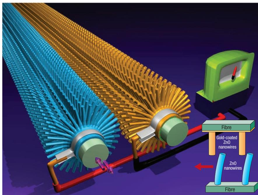
**Figure 1** When ambient vibrations move a microfibre covered with zinc oxide nanowires (blue) back and forth with respect to a similar fibre that has been coated with gold (orange), electrical energy is produced because ZnO is a piezoelectric material.
