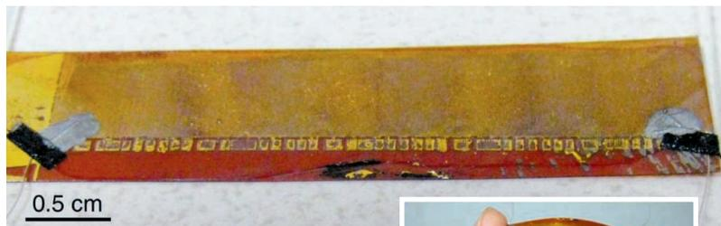
**Good vibrations.** Zinc oxide (ZnO) nanowires are grown between chromium (Cr) and gold (Au) electrodes (top) to make a nanogenerator that produces a high voltage when flexed.
