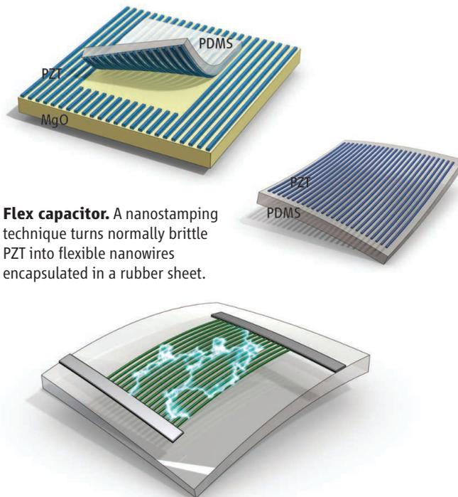
**Flex capacitor.** A nanostamping technique turns normally brittle PZT into flexible nanowires encapsulated in a rubber sheet.
