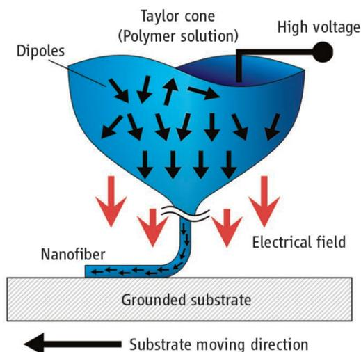
**Power threads.** A large electric field orients electric dipoles in a polymer being drawn into fibers.
