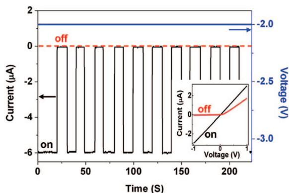
**Figure 5.** Current response of Device no. 4 to periodic releasing-bending process under a fixed bias of  $-2$  V, showing an “on”–“off” ratio of  $\sim 120$ . Inset is  $I$ – $V$  characterization of Device no. 4 without (black curve) and with stain (red curve).
