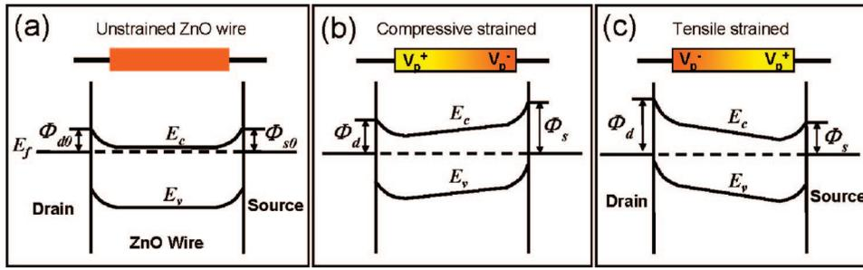
**Figure 4.** Schematic energy band diagrams illustrating the Schottky barriers at the source and drain contacts of an unstrained (a), compressive strained (b), and tensile strained (c) PFW, which illustrates the effect of switching the piezoelectric potential either by strain or by wire orientation on the local band structure and SBH.
