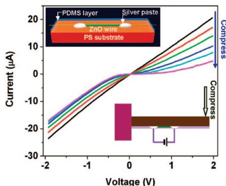
**Figure 1.** Typical  $I$ – $V$  characteristics of the device under different compressive strains (Device no. 1). Black line is the  $I$ – $V$  curve without strain. The direction of the blue arrowhead indicates the increase of applied compressive strain. Upper inset shows the schematic of a single ZnO PFW-based device. Lower inset shows the schematic of the electromechanical measurement system.
